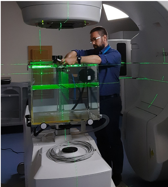
Radiotherapy physics clinical scientist performing commissioning checks on a radiotherapy linear accelerator treatment machine using a scanning water tank.
