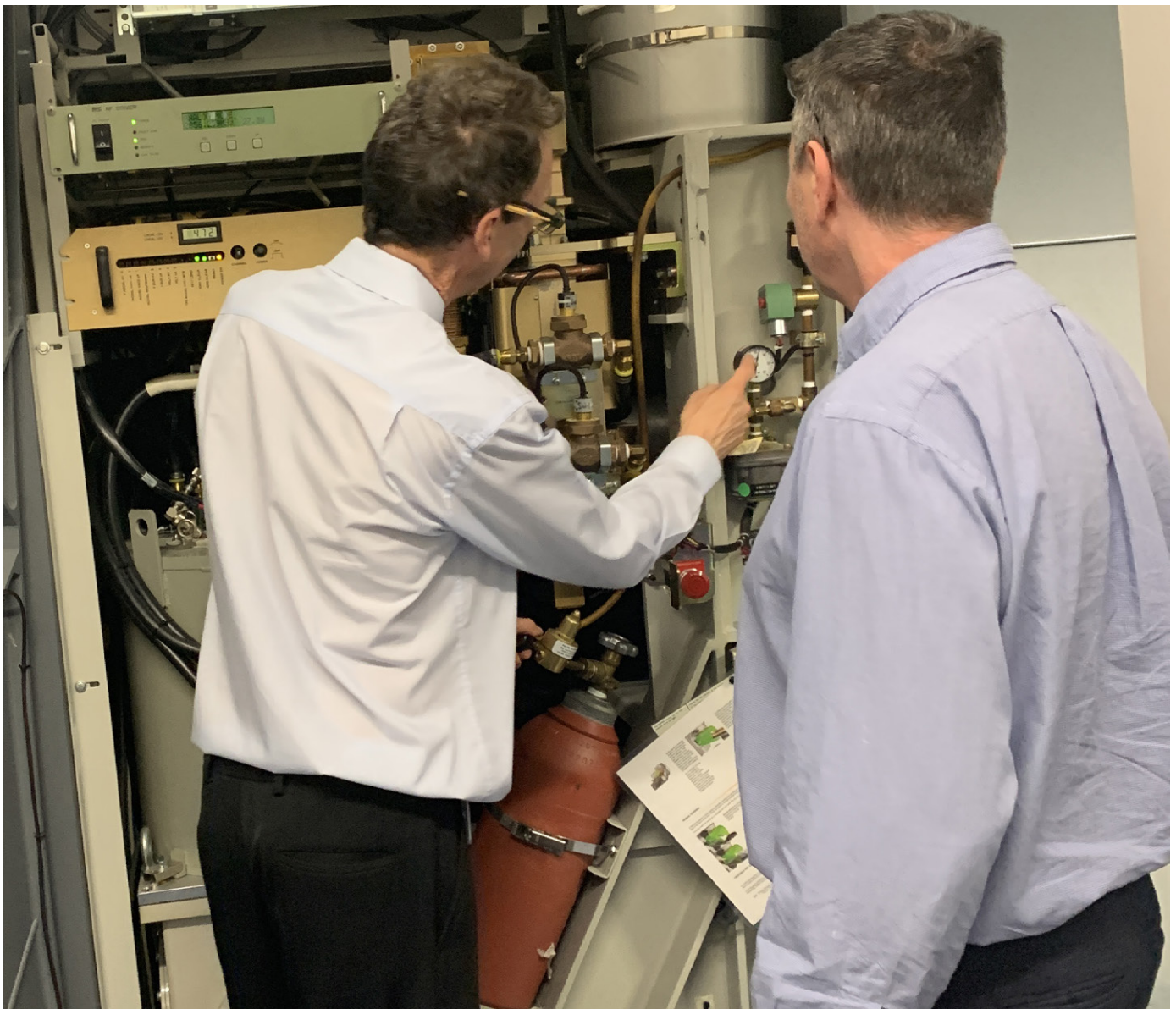
Radiotherapy clinical technologists inspecting components of a radiotherapy linear accelerator treatment machine
